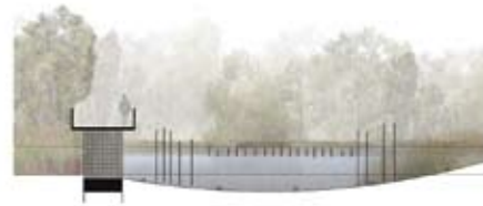
Trattamento terziario Le piante fitodepurative ed il terreno filtrano i microrganismi e digeriscono i nutrienti Tertiary treatment Wetland plants and soils filter microorganisms and digest nutrients
