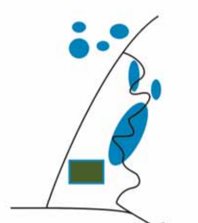
Flood storage in sequence of detention ponds Forested zone for overflow flooding
