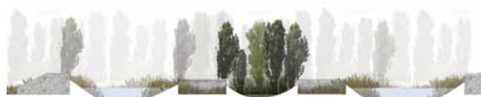
riverine marsh: final filtration and disinfection occurs in deep polishing ponds
